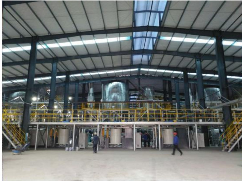
Project3 sets of PSD-60 Large Precision Spray Dryer for Battery Materials in Hunan Province
